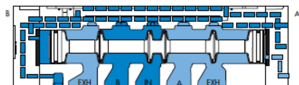
2 POSITION SINGLE PRESSURE SHOWN WITH "B" OPERATOR ENERGIZED
